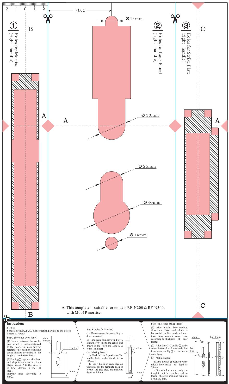
Remarks: 1. Position and size of the holes must be confirmed before cutting. 2. If there is shock absorption bar on door frame, its thickness should be excluded from door thickness.
