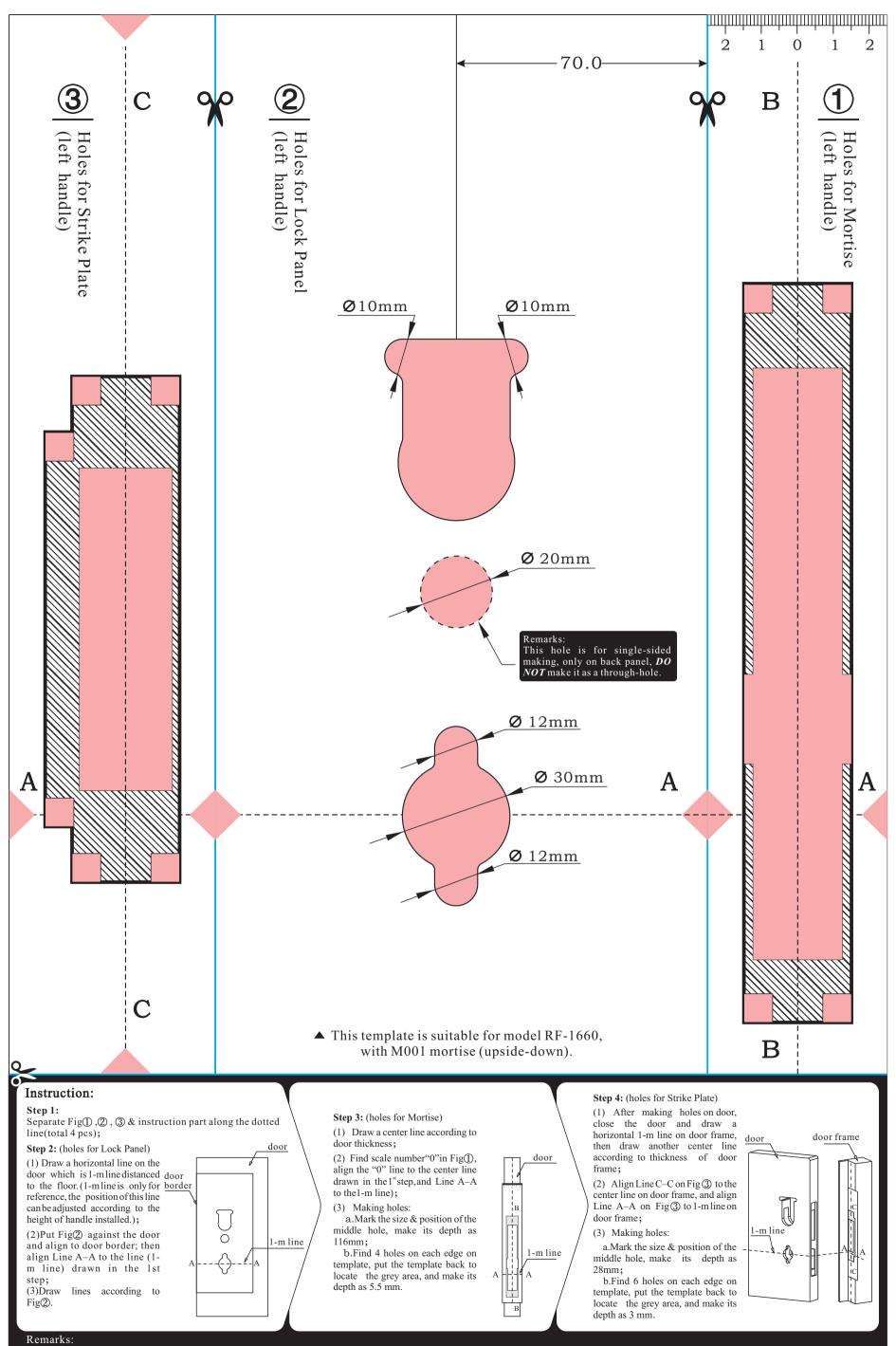
1. Position and size of the holes must be confirmed before cutting. 2. If there is shock absorption bar on door frame, its thickness should be excluded from door thickness.
